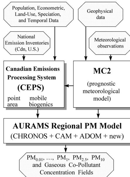
**Figure 1** Schematic diagram of AURAMS building blocks.
