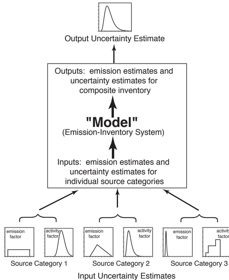
**Figure 8.2. Conceptual Framework for Propagation of Uncertainty in Emission Inventory Inputs of Emission and Activity Factors for Each of  $k$  Emission Source Categories to Quantify the Uncertainty in the Estimate of Total Emissions.** A variety of probability distribution models can be specified to represent uncertainty in inputs.
